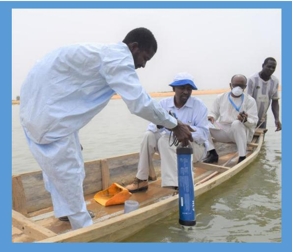
Field measurements of water quality by LCBC experts using a modern sonde provided by UNESCO for calibration and validation of satellite-derived data on the UNESCO World Water Quality Portal
