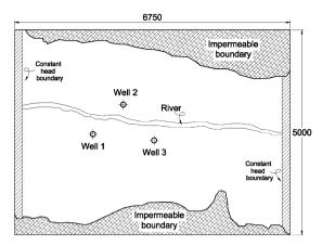
Fig. 4. Modeling domain for the three layer model; adapted from Chiang (2001).
