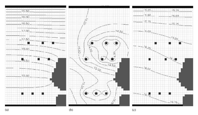
Fig. 6. Simulated heads obtained with PMWIN for case 1: (a) steady state simulation heads; (b) transient heads for stress period 1, time step 12; and (c) transient heads for stress period 12, time step 6.
