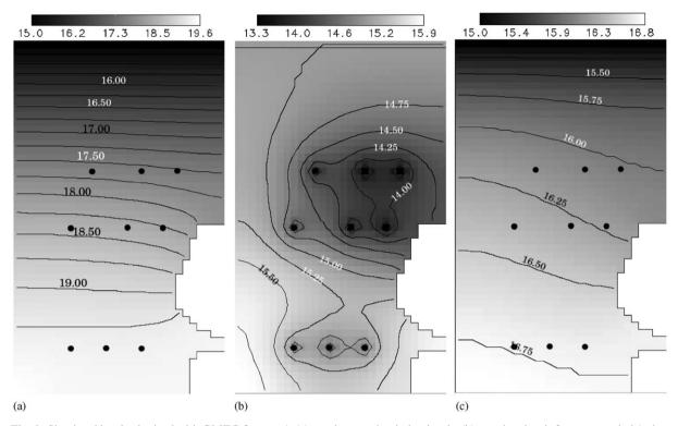
Fig. 5. Simulated heads obtained with GMTG for case 1: (a) steady state simulation heads; (b) transient heads for stress period 1, time step 12; and (c) transient heads for stress period 2, time step 6.
