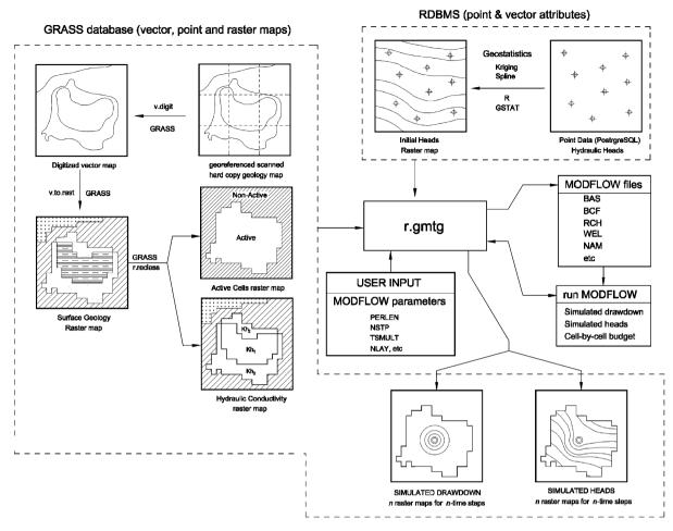
Fig. 2. Interaction of r.gmtg with GRASS and MODFLOW.
